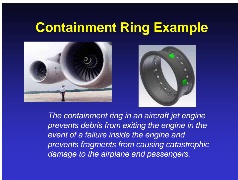
Figure 7. Jet engine containment ring problem
